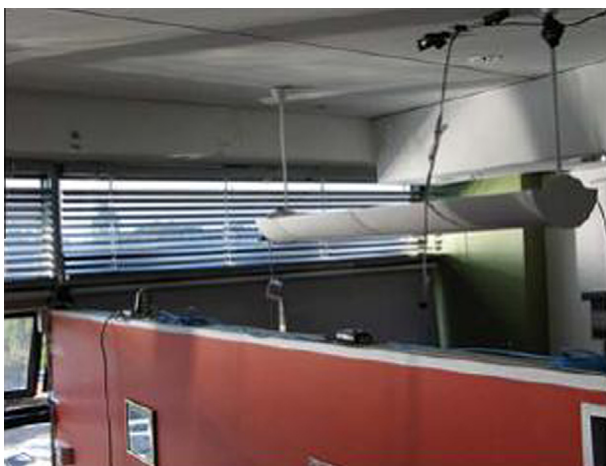
Fig. 7. Lux meter sensors in horizontal position on top of partition wall.
